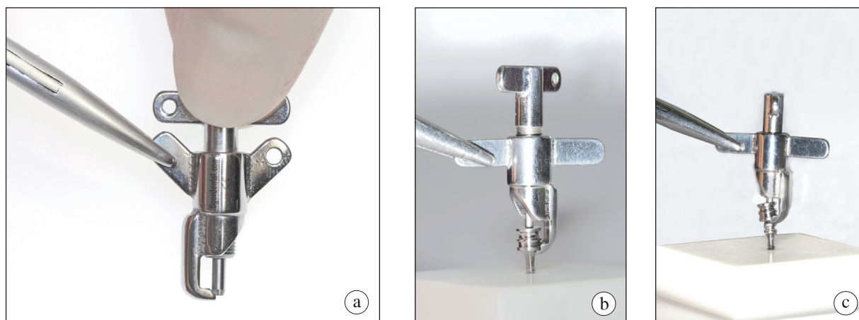
Fig. 9. The collar extractor designed for removing the collars from the implant heads.
